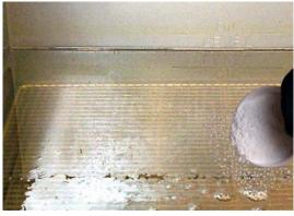
Adding filter powder to vat prior to filtering.
